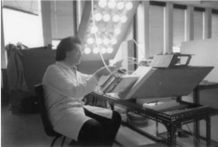
Fig. 3. Connecting the K-thermocouples to the water-heater.
