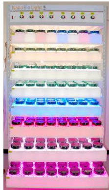
Fig. 2. Tissue culture cart developed (Left: Giant E-Light, 8 layers, 40 vessels per layer, L107-W62-H195 in cm, power consumption: 110VAC/12A or 220VAC/5.5A; Right: Mini E-Light, 2 layers, 12 vessels per layer, L66-W40-H80 in cm, power consumption: 110 VAC/0.61A or 220VAC/0.3A).
