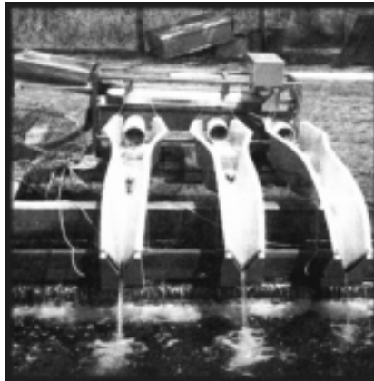
The Fischtechnik FGM4 Grader working in unison with the Vaki Bioscanner System 3
