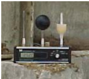
Figure 8. The heat stress monitor (hs-3600, Metrosonics, INC.). From the left, there are dry bulb, black globe and wet bulb temperature probes.
