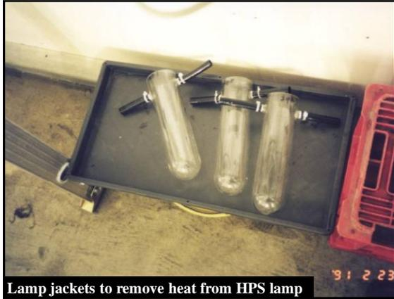
Lamp jackets to remove heat from HPS lamp
