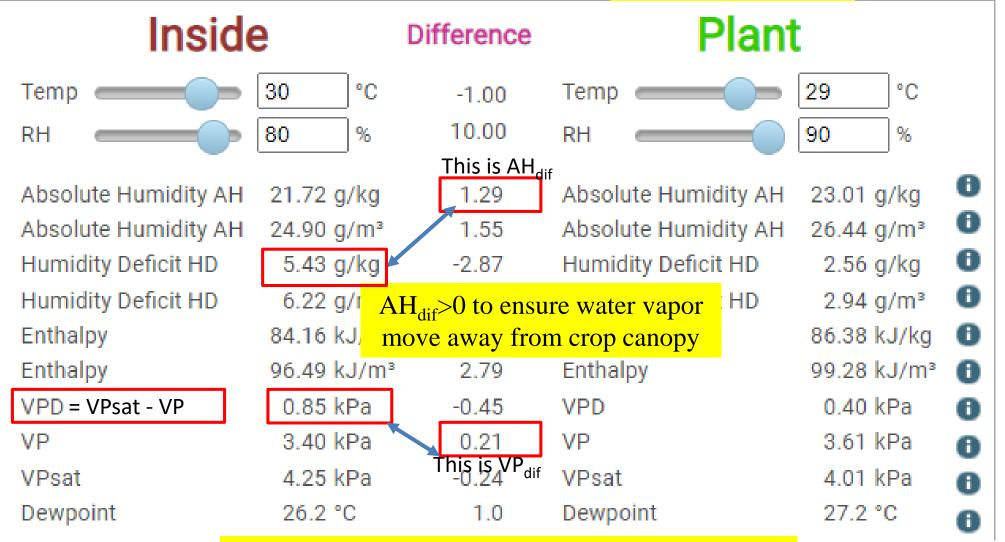
AHD is not equal to AH<sub>dif</sub>, AHD is the AH@Tsat – AH@Tdb VPD is not equal to VP<sub>dif</sub>, VPD is the VP@Tsat – VP@Tdb
