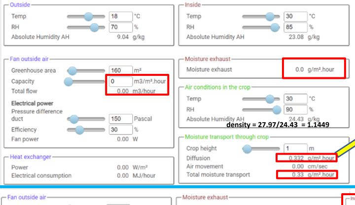
When fan capacity =  $0 \text{ m}^3/\text{m}^2.\text{h}$ , There is no air exchange between in & outdoor, thus, Moisture exhaust = 0
