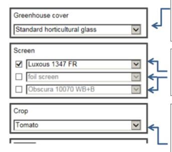
Here you can select an appropriate greenhouse cover. The list contains a number of typical greenhouse coverings, ranging from glass to poly coverings and can be single or double. For each of the coverings the model uses typical properties for its transmissivity for solar radiation, convective exchange and its transmissivity for thermal radiation.
