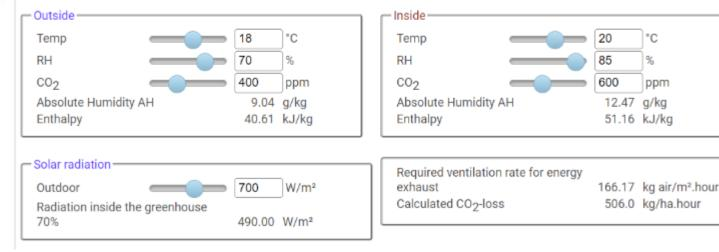
Qin = (700 \* 0.7 \* 3.6) in kJ/m<sup>2</sup>.h dEnthalpy = (51.16 - 40.61) in kJ/kg Vent. rate = Qin / dEnthalpy
