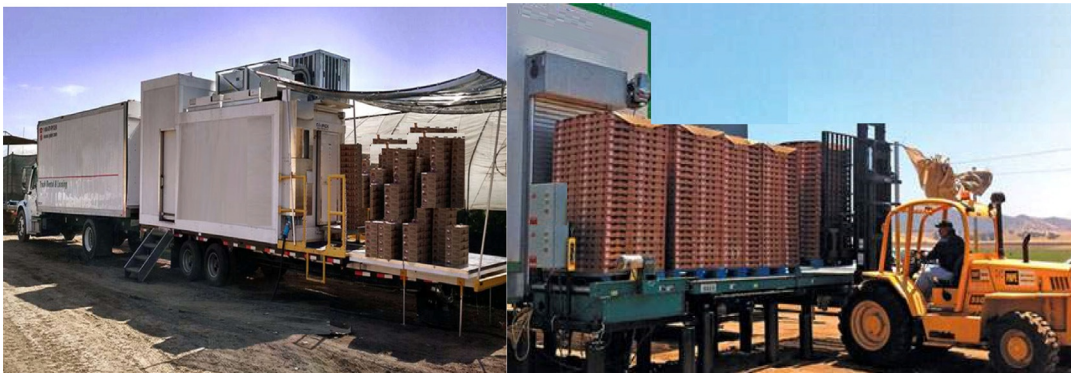
FIG. 6.14 ColdPICK M1 mobile precooling system on the left and Cold@Field mobile precooling system on the right.
