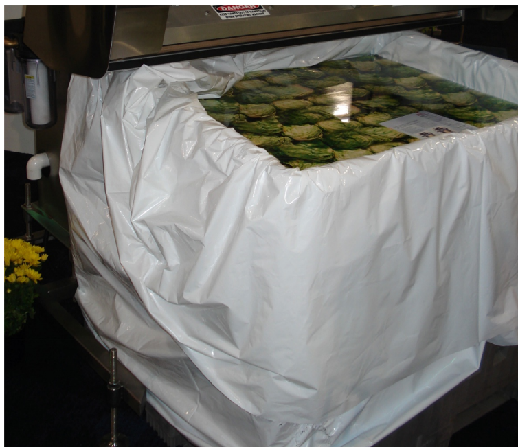
FIG. 6.18 Hydrocooler with water/ice mixture for small scale operation.
