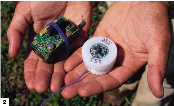
NOTHING BUT NET: John Anderson [1] buries a mote [2, two variants shown] in the dirt wall of a petrel burrow. Other motes nearby on thin wire stalks [3] monitor the weather.
