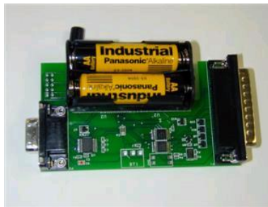
Fig. 3. MICA2 base station mote
