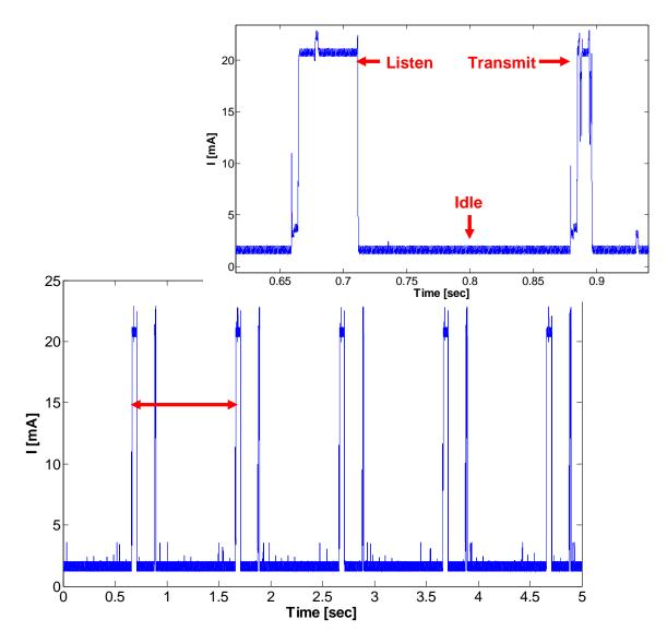
Figure 10. Actis current consumption during 5 seconds of operation. Red arrow marks one super frame cycle.
