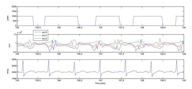
Figure 3. ECG, acceleration, and foot switch data collected by the WWBAN prototype during normal walking.
