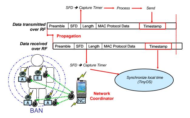
Figure 8. Time Synchronization in WBAN prototype.
