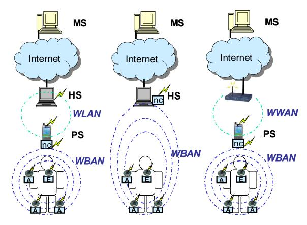
**Figure 2. WWBAN Deployment Scenarios.** Legend: A – Activity Sensor, E – Heart Sensor, WBAN – Wireless Body Area Network, PS – Personal Server, WLAN – Wireless Local Area Network, WAN – Wide Area Network, HS – Home Server, MS – Medical Server, nc – WBAN network coordinator.
