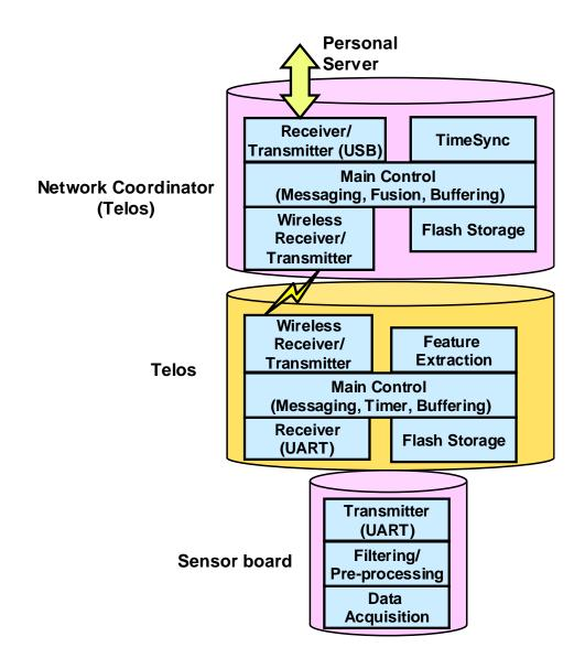
Figure 6. WBAN Software Architecture.
