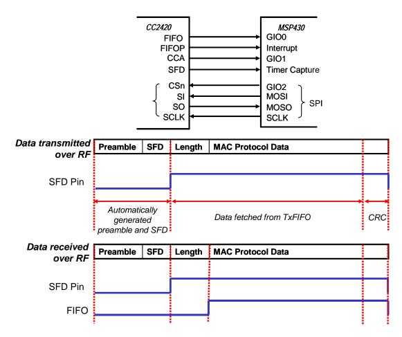
Figure 7. Interfacing CC2420 RF transceiver (top). IEEE 802.15.4 frame format and pin
