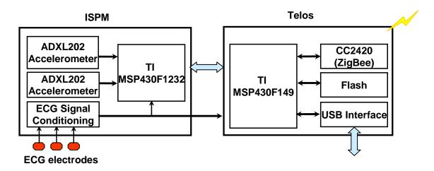
Figure 5. Block diagram of an ActiS sensor node.
