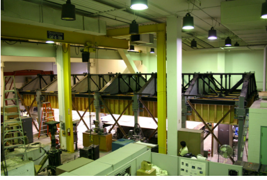
Figure 4: The seismic test structure
