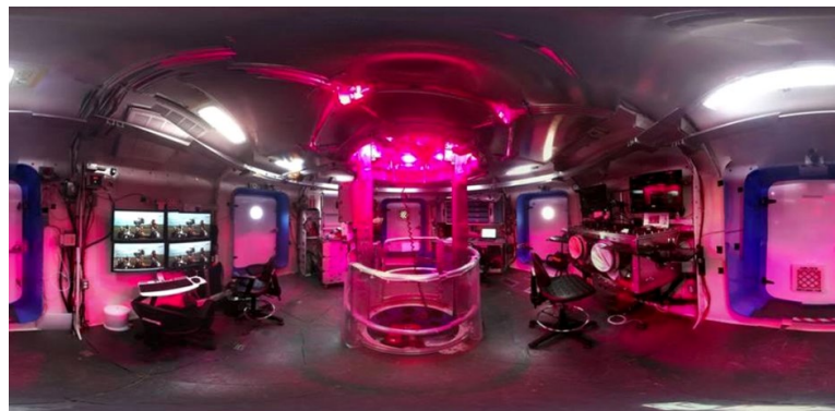
Fig. 3. Wide angle view of NASA's Habit Demonstration Unit work laboratory showing effect of red/blue LED's positioned in plant atrium.
