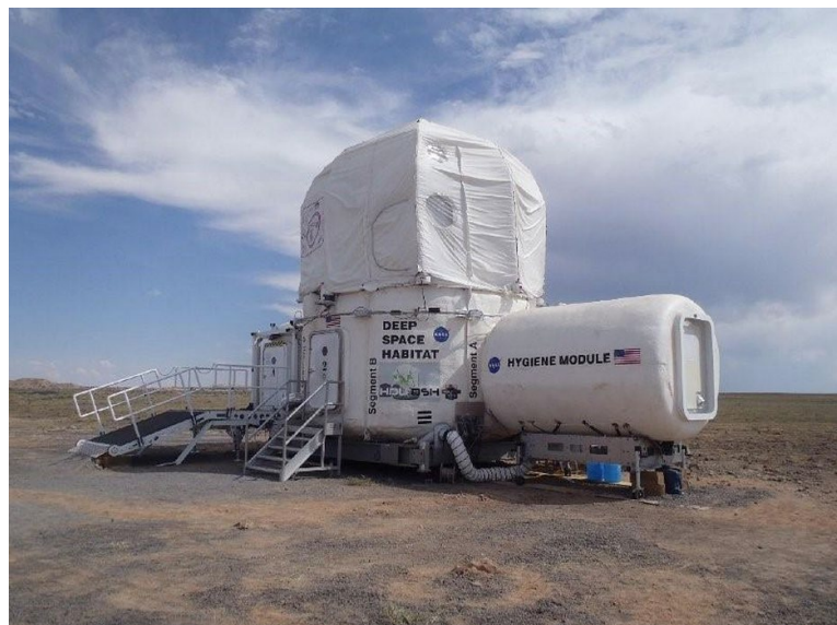
Fig. 2. NASA's Deep Space Habitat Module on location for field testing in Arizona Desert. A food production system was integrated as an atrium between the living (upper) and working (lower) areas.
