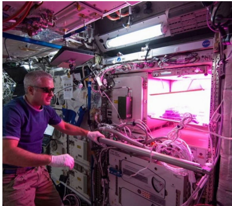
Fig. 1. International Space Station crew member, Dr. Steve Swanson tending the Vegetable Production System (Veggie) on ISS during Expedition 40. Veggie is a plant growth system installed on ISS which uses a LED lighting system that is designed to produce salad-type crops to provide the crew with fresh food while on orbit. (Photo courtesy of NASA Public Affairs Office).
