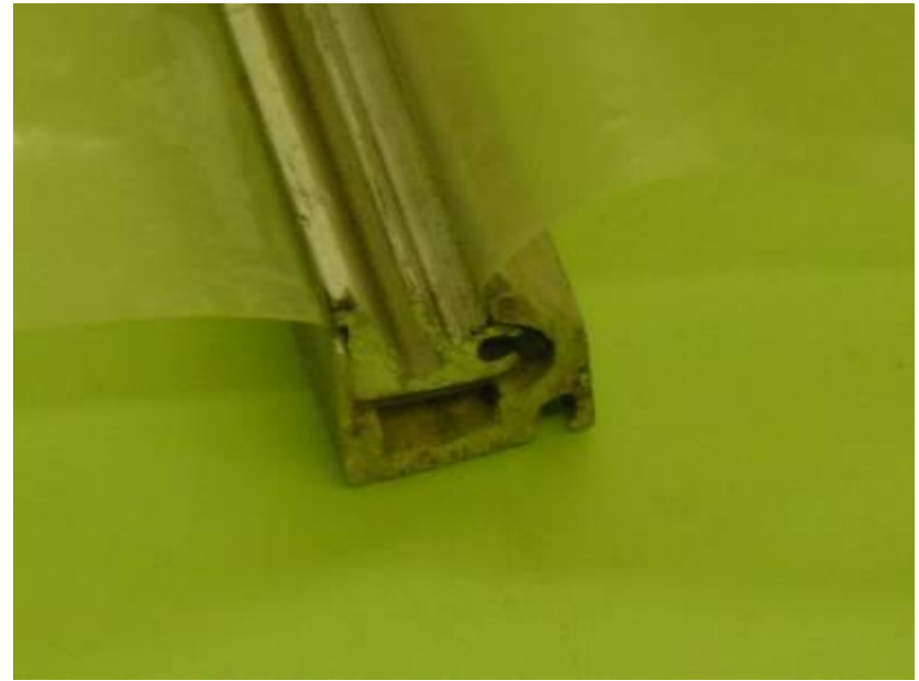
Fasteners evolved from simple wood nailers to engineered extrusions
